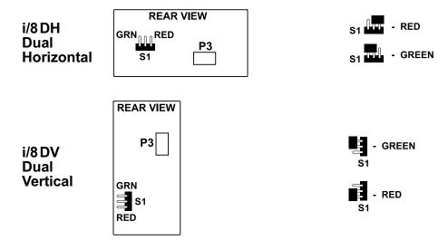
Figure 2.14 i/8D Location of S1 and Selectable Jumper Positions
